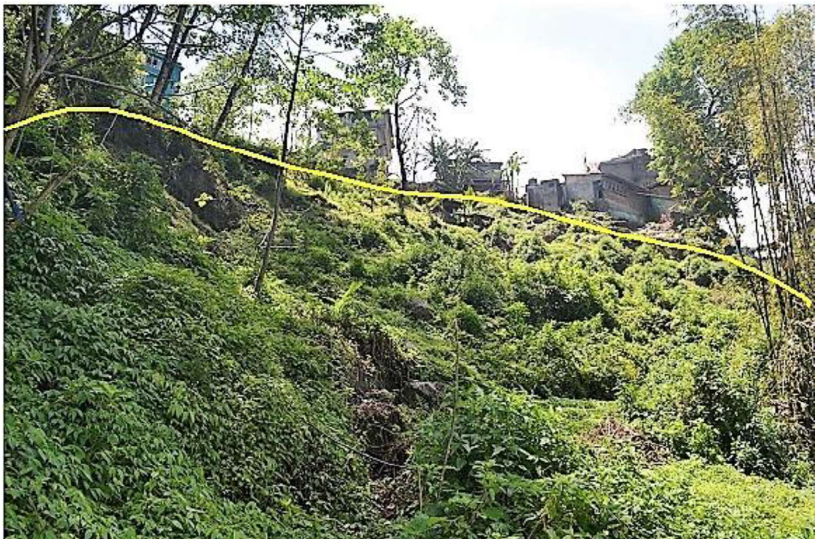
Fig 7: Showing crown portion of the slide zone below SNT complex.
